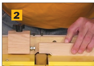
Pass 2 - Clean out the side of the notch.
