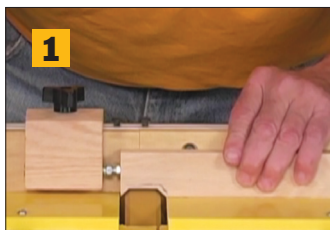
Pass 2 - Clean out the side of the notch.
