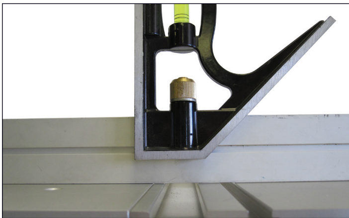
Photo above shows proper alignment of the top and is flat
