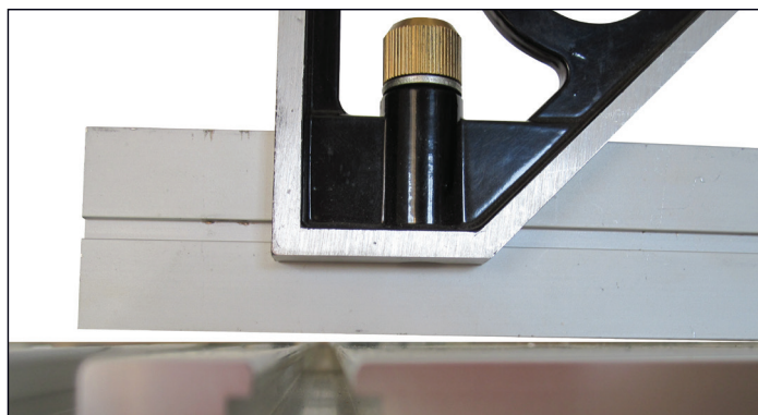
Photo above shows improper alignment of the top and is not flat
