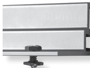
Thread the 1/4" weld nuts loosely onto the 5/16" x 1-1/2" hex bolts
